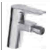
HANSATWIST one-hole single-lever mixer, DN 15 for bidet 0906 3283 chrome Solid lever (Metall), pop-up waste (metal), connection with flexible pressure hoses projection: 112 mm
