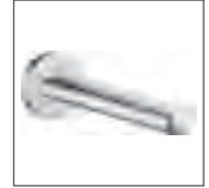
HANSAARONDA bathtub spout, DN 15 (G 1/2)** 0582 2172 chrome also compatible with HANSAMATRIX projection: 180 mm
