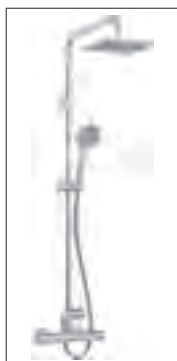
HANSAUNITA thermostatic shower mixer, DN 15 (G 1/2) 5814 9113 0067 chrome with shower system directly connected, shower head square 200 x 200 mm, HANSAVIVA hand shower, 100 mm, 3-spray
