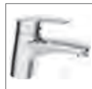
HANSAMIX one-hole single-lever basin mixer, DN 15 0118 2183 chrome without pop-up waste, spout: swivel, connection using copper pipes projection: 157 mm
