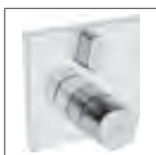
HANSABLUEBOX function unit with trim kit HANSA|LIVING bath thermostatic mixer, DN 15 (G1/2) with integrated ceramic volume regulation with vacuum breaker * 8114 3562 chrome rosette without screws, squared rosette, 150 x 150 mm, function unit with BLUESWITCH diverter and volume control
