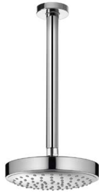
51684 Shower head with ceiling-outlet DN 15 Ø 180 mm, with shower head rail, restricted flowrate 10 l/min., Height: 100, 300 mm
