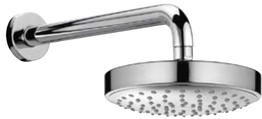
51683 Shower head with wall-outlet DN 15 Ø 180 mm, with shower head rail, restricted flowrate 10 l/min., Projection: 300, 450 mm
