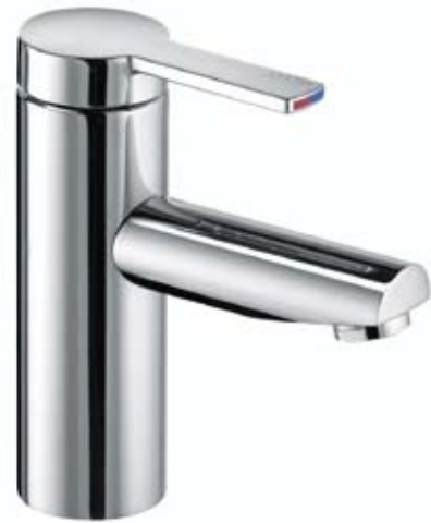
53902 Single lever basin mixer with/without pop-up waste, 1-hole installation, cartridge mixer with ceramic sealing gaskets and temperature limiter, restricted flow rate 6 l/min. Height: 161 mm Projection: 144 mm
