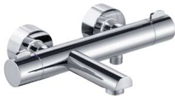
53920 Bath tub mixer DN 15 exposed Cartridge mixer with ceramic sealing gaskets, restricted flow rate 12 l/min., ceramic stop valve and diverter, wall outlet for shower hose DN 15, restricted flow rate 12 l/min., gauge 150 +/- 14 mm Width: 310 mm Projection: 222 mm
