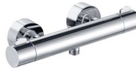
53924 Shower mixer DN 15 exposed ceramic stop valve, Cartridge mixer with ceramic sealing gaskets, wall outlet for shower hose DN 15, restricted flowrate 12 l/min., gauge 150 +/- 14 mm Width: 311 mm Projection: 104 mm
