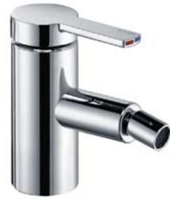
53909 Single lever bidet mixer with pop-up waste, 1-hole installation, cartridge mixer with ceramic sealing gaskets and temperature limiter, restricted flow rate 6 l/min. Height: 136 mm Projection: 138 mm
